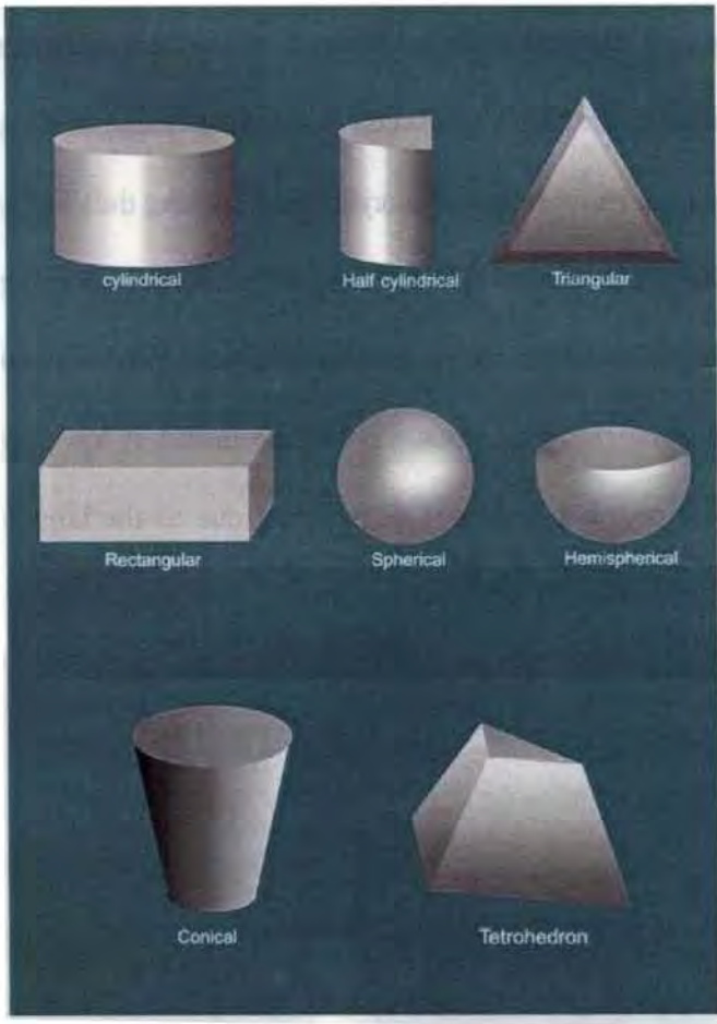
Fig. 1.2 Various geometries of DRAs
