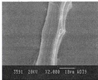
Figure 1.20. SEM photograph of a single fibril of isora fibre
