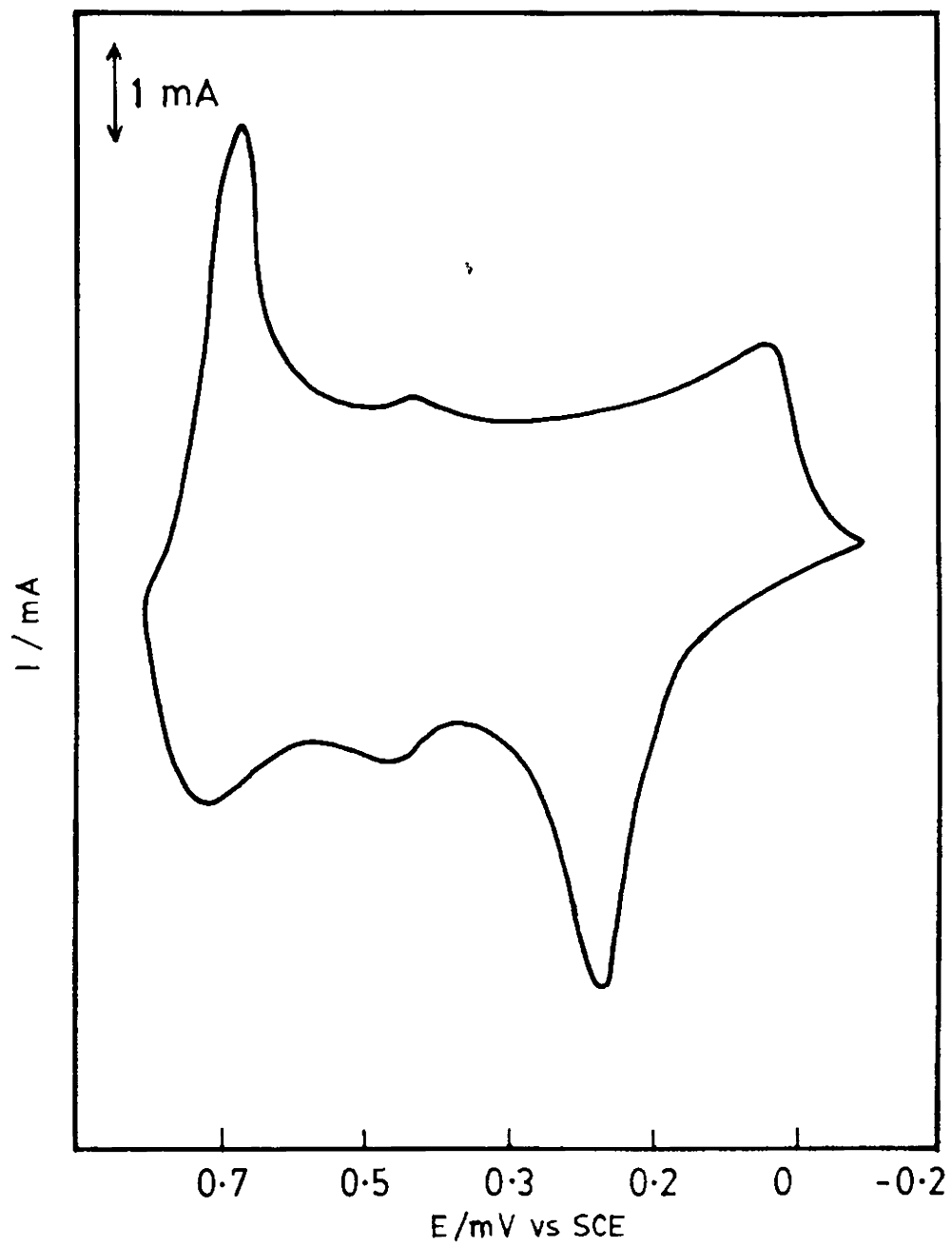
Fig. 5.4 Cyclic voltammetric behaviour of PA film deposited on platinum electrode. Supporting electrolyte : 0.5M \text{H}_2\text{SO}_4
