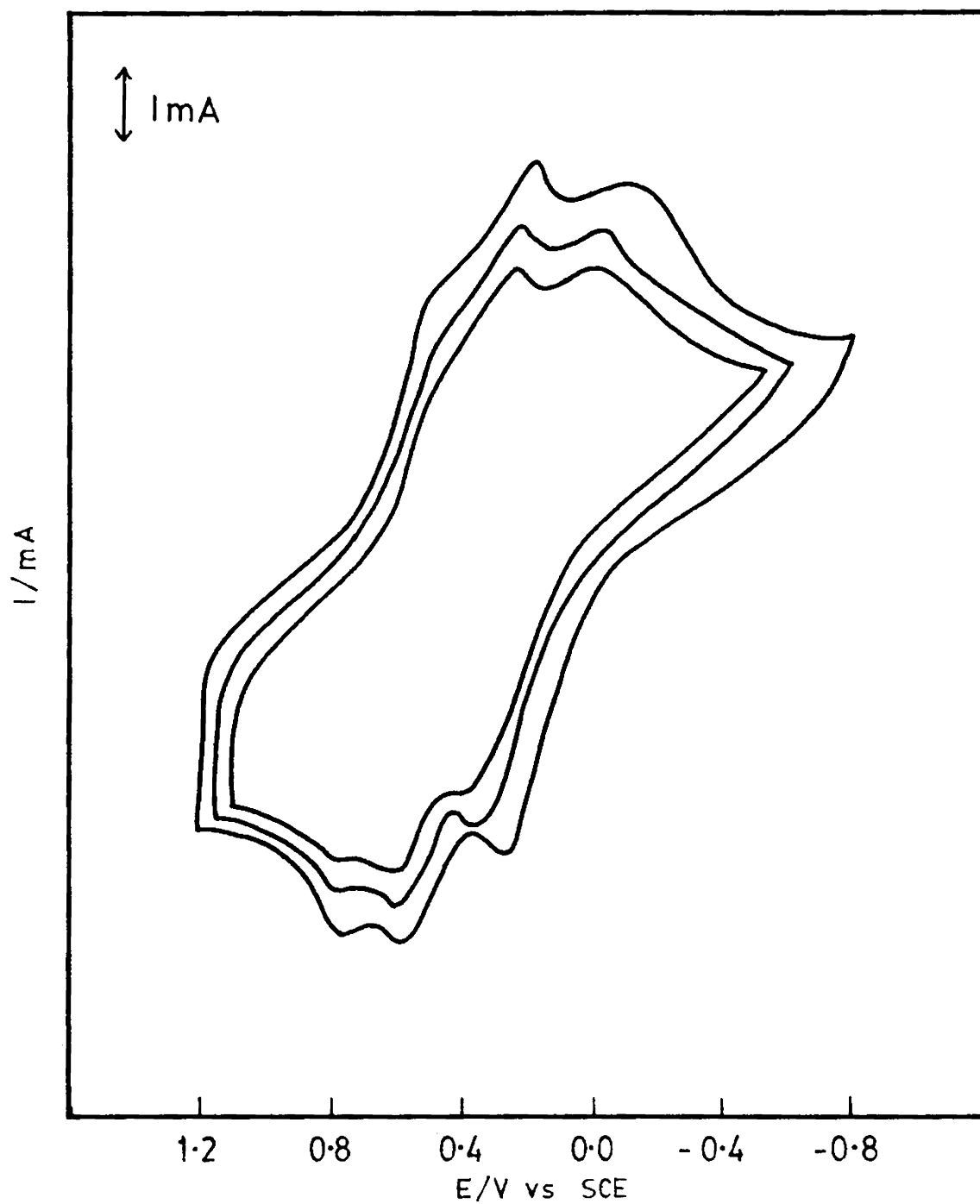
Fig. 5.5 Cyclic voltammetric behaviour of chemically prepared polyaniline-carbon paste electrode. Supporting electrolyte : 0.5M \text{H}_2\text{SO}_4 Scan rate : 100mV/s
