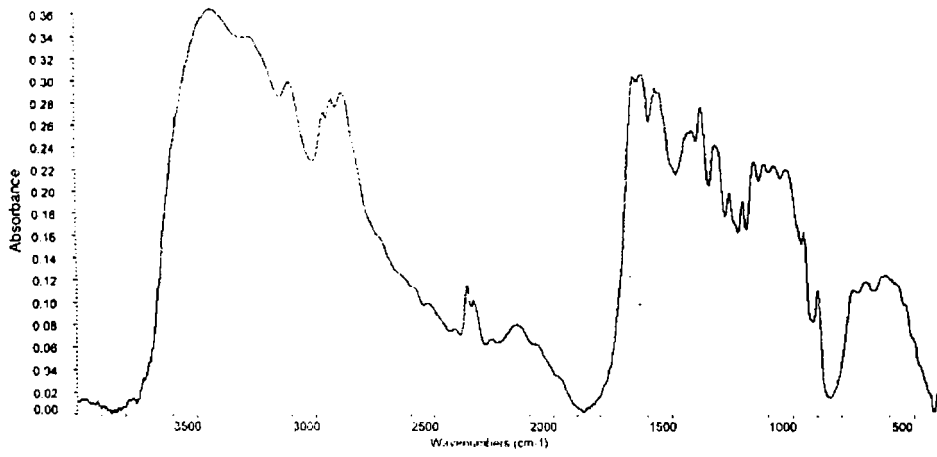
Fig. 5 b. FTIR spectrum of chitin prepared from lactic acid treated shell residue
