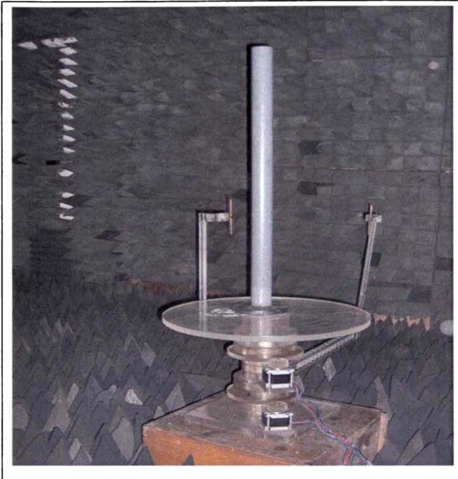
Figure 6.25 The measurement setup in the anechoic chamber facility of DOE, CUSAT
