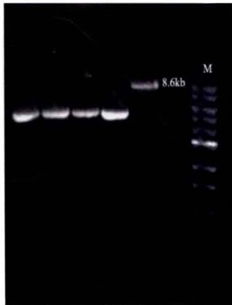
Fig.4. Agarose gel showing the vector pSV3-neo isolated from E. coli HB101 (lanes 1-4), vector linearised with Eco RI (lane5) (M- 1kb ladder)
