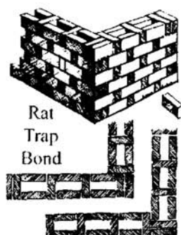
Figure 5.1 Schematic representation of rat trap bond masonry (Source: Baker, 1993c)
