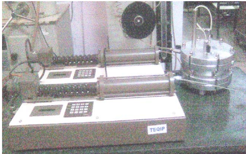
Fig 3.12 Experimental setup for Permeability Measurement using Rowe Cell Apparatus
