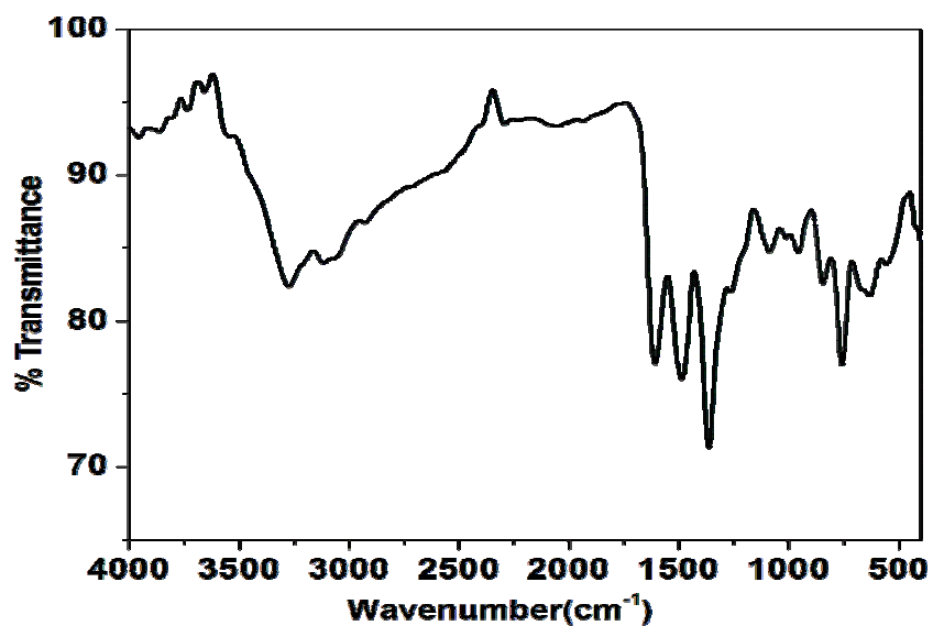
Figure 6.3. FTIR spectrum of [Cu(qc6in)Cl 2 ]
