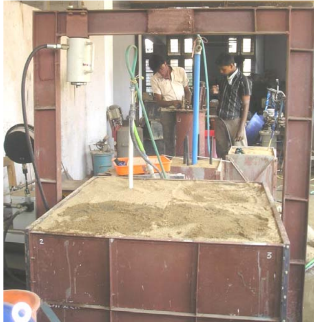
Fig. 5.5(b). Grouting process in large tank in progress
