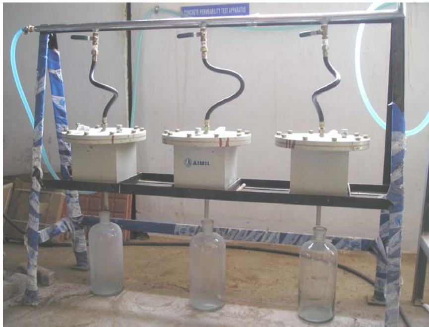
Fig. 3.6 Permeability test set up for grouted samples.
