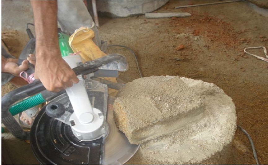
Fig. 3.4 (a) Collection of test specimens from grouted samples in progress
