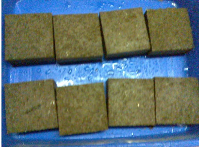
Fig 3.3 Samples for direct shear test
