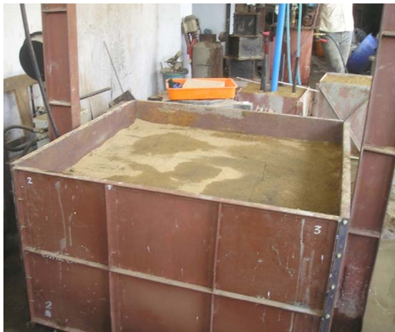
Fig. 5.6 Grouted sand bed
