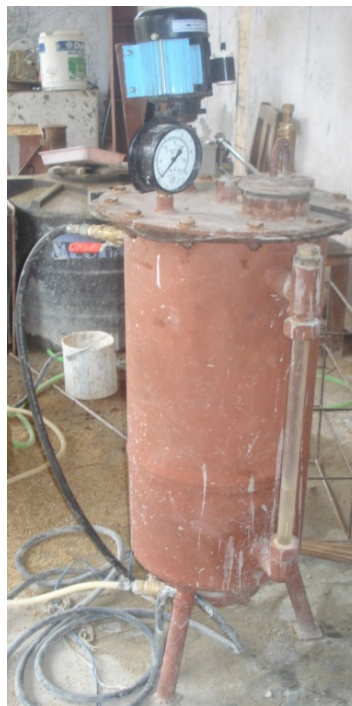
Fig.5.1 (b) Grout chamber
