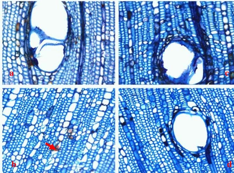
**Figure 4. 3. Light microscopic image of CCA treated panels with retention of  $29 \text{ kg m}^{-3}$**
