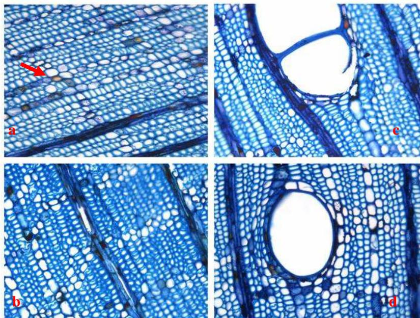
**Figure 4. 4. Light microscopic image of CCA treated panels with retention of  $42 \text{ kg m}^{-3}$**
