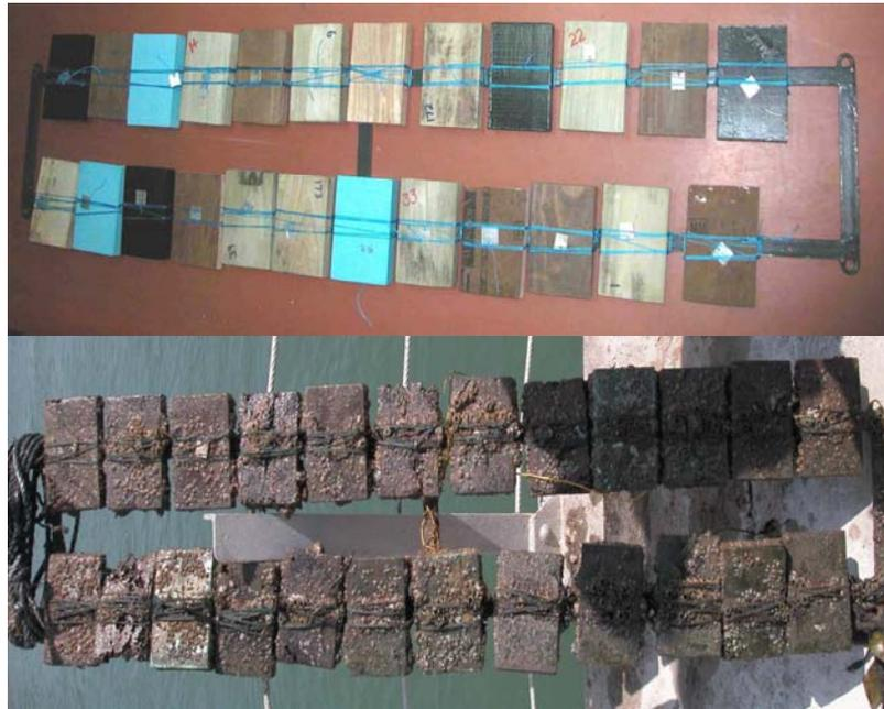
**Figure 9.1. a) Panels after immersion in the Cochin estuarine waters for 18 months b) a close view of foulers on the panels**
