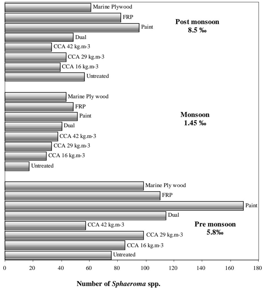
Figure 9. 3. Major biofouling organisms observed on the panels
