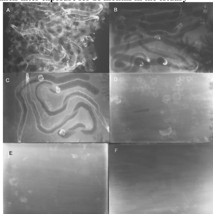
\*A. untreated rubber wood, B. Marine plywood, C. CCA treated (16 kg m<sup>-3</sup> retention), D. CCA treated (29 kg m<sup>-3</sup> retention), E. CCA treated (42 kg m<sup>-3</sup> retention) F. Dual
