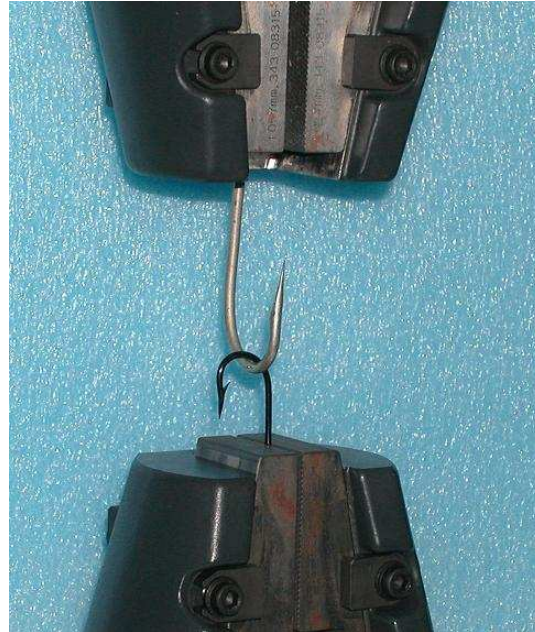
Fig. 5.1. Unbending test of fishing hook using UTM
