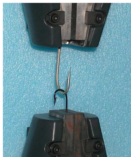
Fig. 2. Unbending test of fishing hook using UTM.
