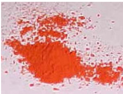
Fig. 14. 20% \alpha\text{-Fe}_2\text{O}_3 , 80% \text{CeO}_2 heat treated at 800°C for 2 h in air atmosphere.
