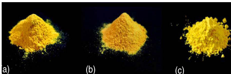
Fig. 17. Representative photographs of the samples: (a) amorphous Ce_{0.8}Zr_{0.2}W_2O_8 , (b) amorphous Ce_{0.8}Ti_{0.2}W_2O_8 , and (c) commercial praseodymium yellow.
