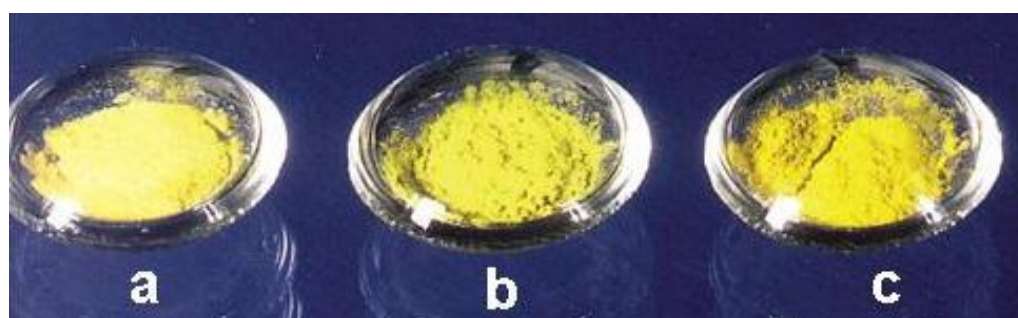
Fig. 16. Colors of (a) CePS 4 , (b) Ce 6 Si 4 S 17 , and (c) Ce 4 Si 3 S 12 .
