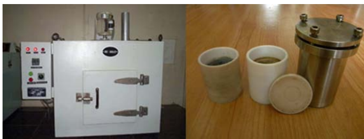
Figure 2.3: Hydrothermal furnace and autoclave used for the synthesis of nanostructures
