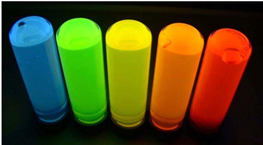
Figure 1.1: Size dependent luminescent emission ranging from blue to red from CdSe quantum dots. On the left is the smaller size quantum dots having blue emission (Image Courtesy of M. S. Wong, Rice University)
