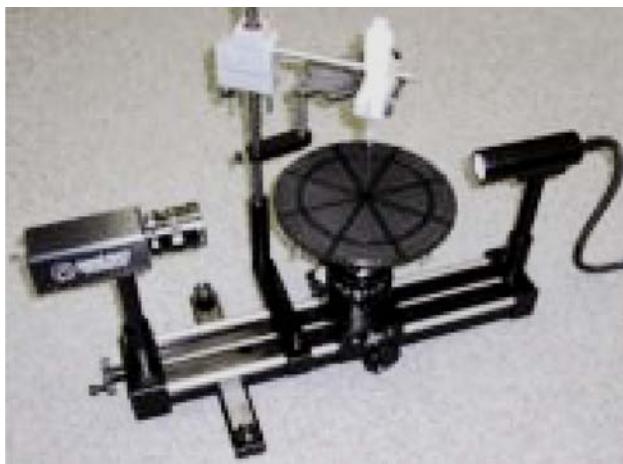
Fig 2.6 A photograph of a standard goniometer
