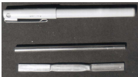
Figure 3.4: Photograph of the bare and powder filled pressed SS tube (L ~ 10 cm, OD/ID = 6/4 mm).
