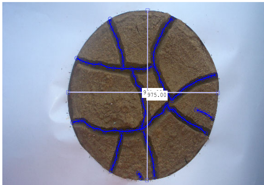
Fig: 4.4 Determination of length of crack
