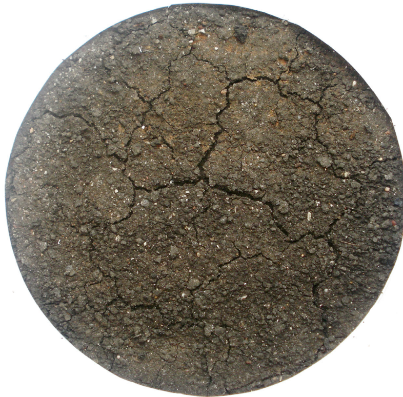
Fig: 4.6 Desiccated Sample of Sundried Marine Clay (Cycle 1)
