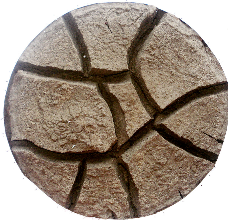
Fig: 4.2 Desiccation cracks in BES sample (Cycle 1)
