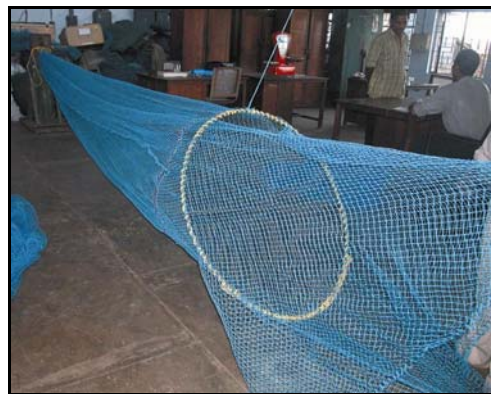
Fig. 8.4. Shrimp trawl codends incorporated with rectangular grid and oval grid
