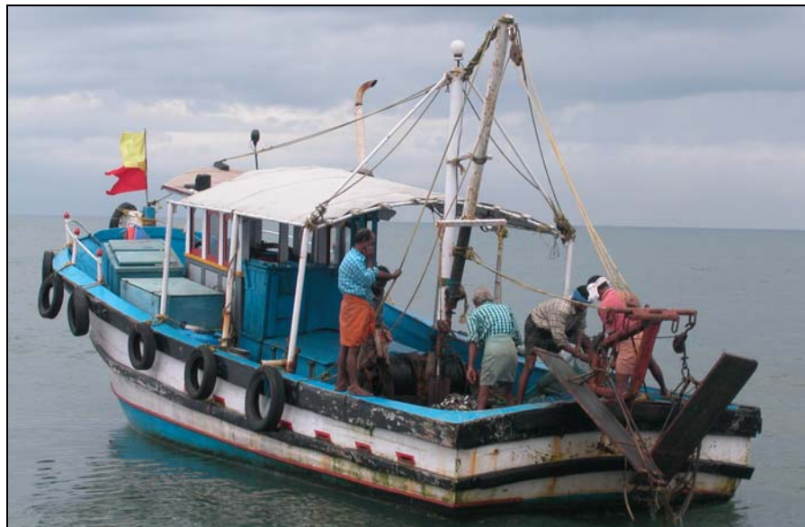
Fig. 4.3. Small trawler with winch
