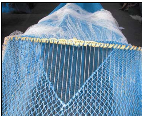
Fig. 8.5. Exit openings before rectangular and oval grid
