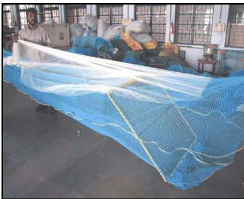
Fig. 8.4. Shrimp trawl codends incorporated with rectangular grid and oval grid
