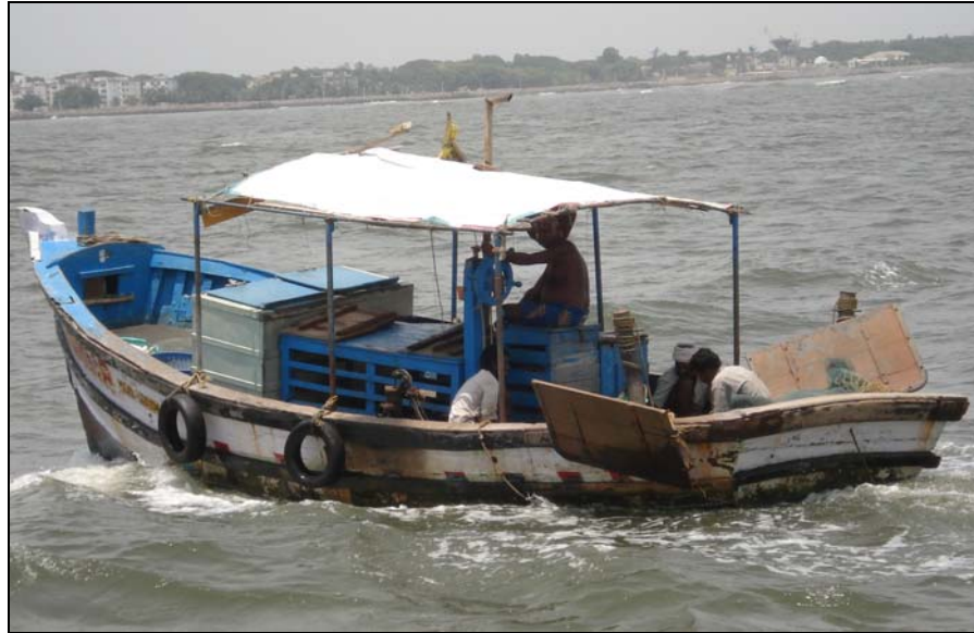
Fig. 4.2. Small trawler without winch
