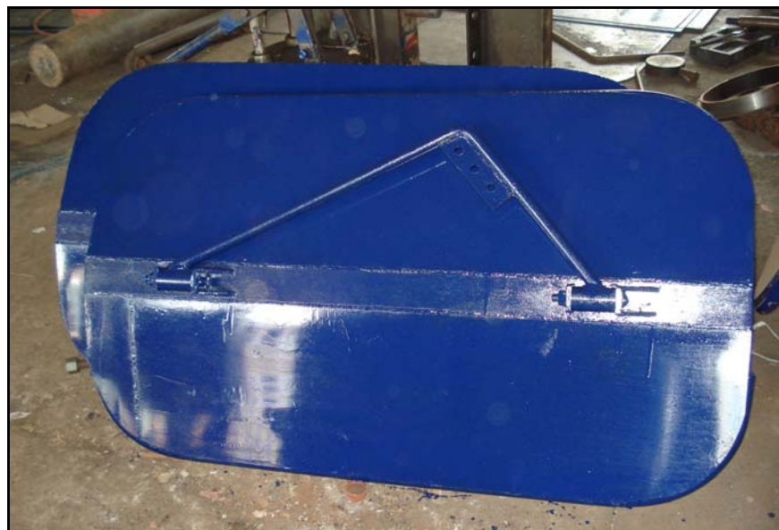
Fig. 4.8. V-type otter board of all steel construction (80 kg)
