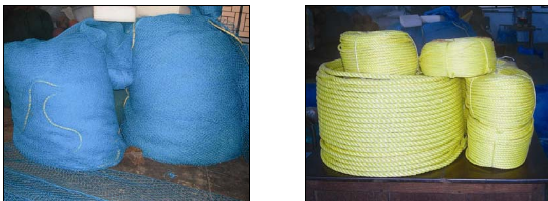
Fig. 4.25. HDPE netting and Polypropylene ropes
