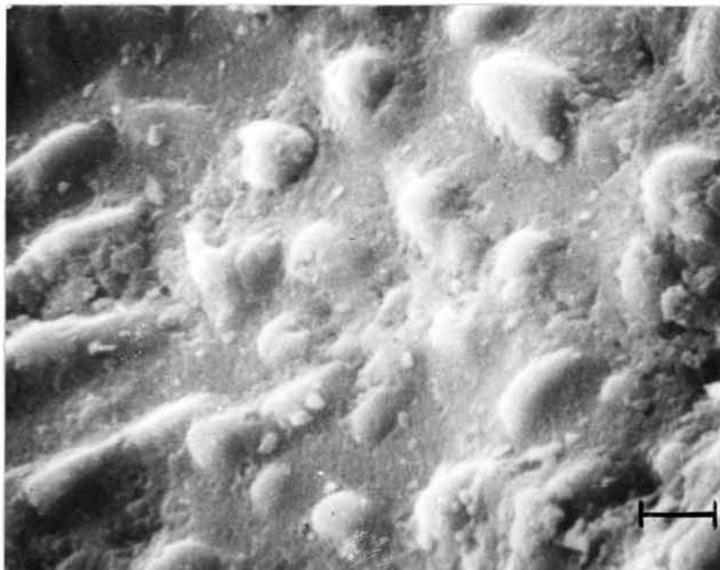
Plate X Superposition of three generations of surface textures on the beach grain. Earlier 'V' pits (a) on the smooth surface of the grain are found to occur with later straight or slightly curved linear grooves (b) The third stage is the formation of widespread silica globules (scale bar 5\ \mu\text{m} )
