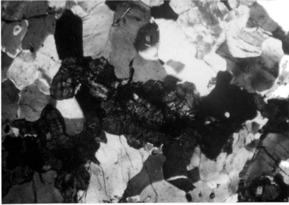
Fig. 21 Photomicrograph showing alteration of pyroxenes preceding that of feldspar in charnockite. Crossed nicol x 25.
