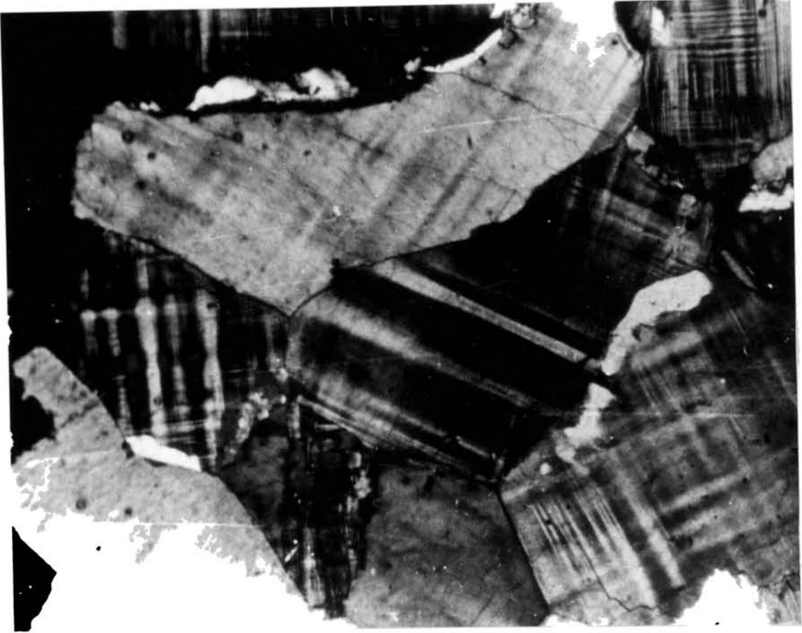
Fig.7 Photomicrograph of microcline in Alkali Syenite showing cross hatched twinning. Crossed nicol x 25.
