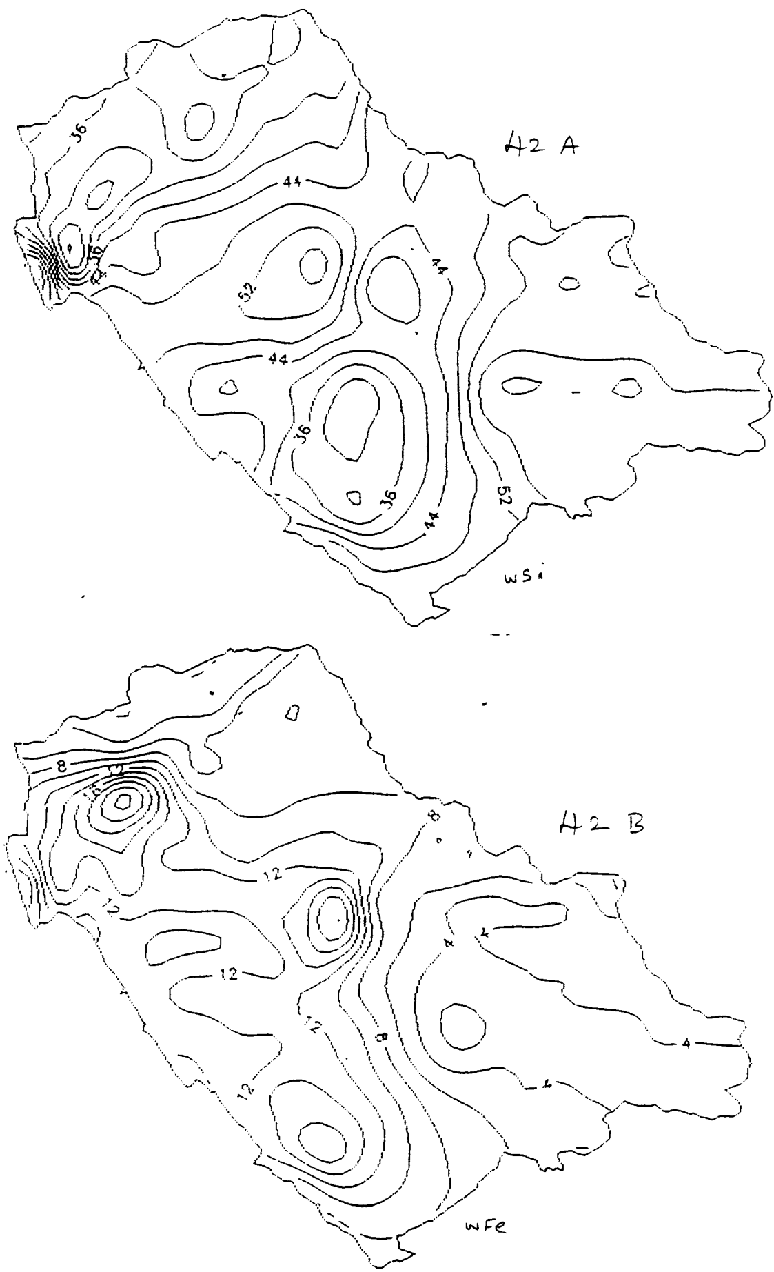
Fig.42 Major element distribution contour maps of Cannanore district based on weathered rock data (42 A : SiO 2 , B : Fe 203 , C : Al 2 O 3 , D : MgO, E : CaO, F : Na 2 O, G : K 2 O, H : TiO 2 , I : LOI.
