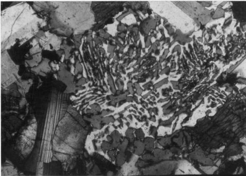
Micropegmatitic intergrowth from the centre of the dyke T 4 ( Scale 1 cm = 0.1 mm).
