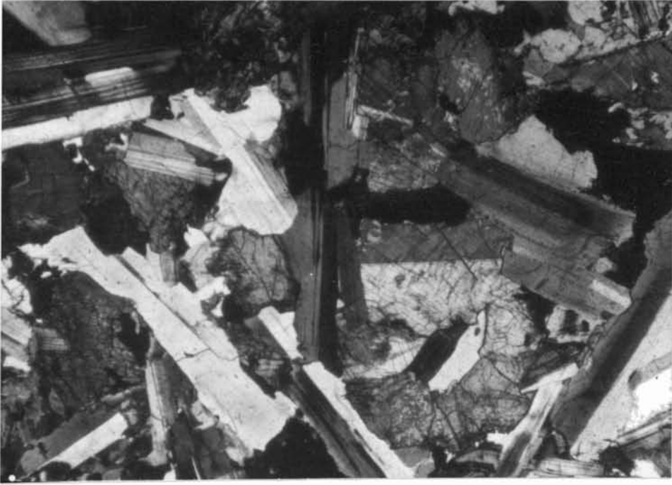
Typical ophitic texture from the centre of the dyke T2 ( Scale 1 cm = 0.3 mm)
