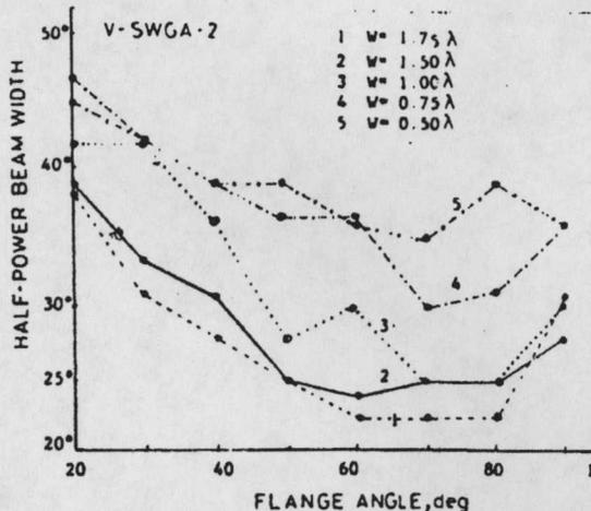
Fig. 6—Variation of half-power beam width against the variation of flange angle for different flange widths
