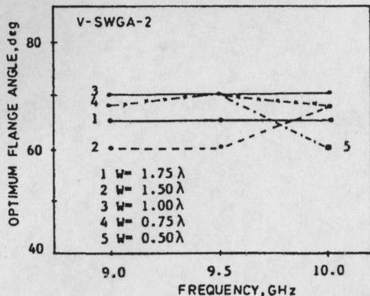
Fig. 5—Dependence of optimum flange angle  $A_0$  on flange width for different frequencies
