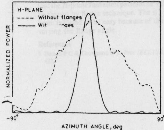
Fig. 3—Typical radiation patterns of V-slot waveguide antenna with and without flanges ( $f = 9.50$  GHz)
