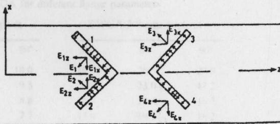
Fig. 1—Electric field variations across the V-slot
