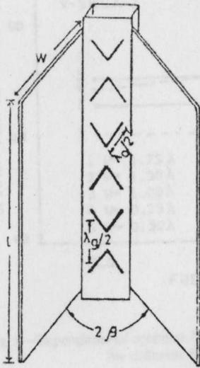
Fig. 2—Schematic diagram of V-slot antenna with flanges ( $W$  = width of the flange,  $l$  = length of flange,  $2\beta$  = included angle of the flange,  $\lambda_0/2$  = length of the arm of V-slot,  $\lambda_0/2$  = separation between two V-slots)
