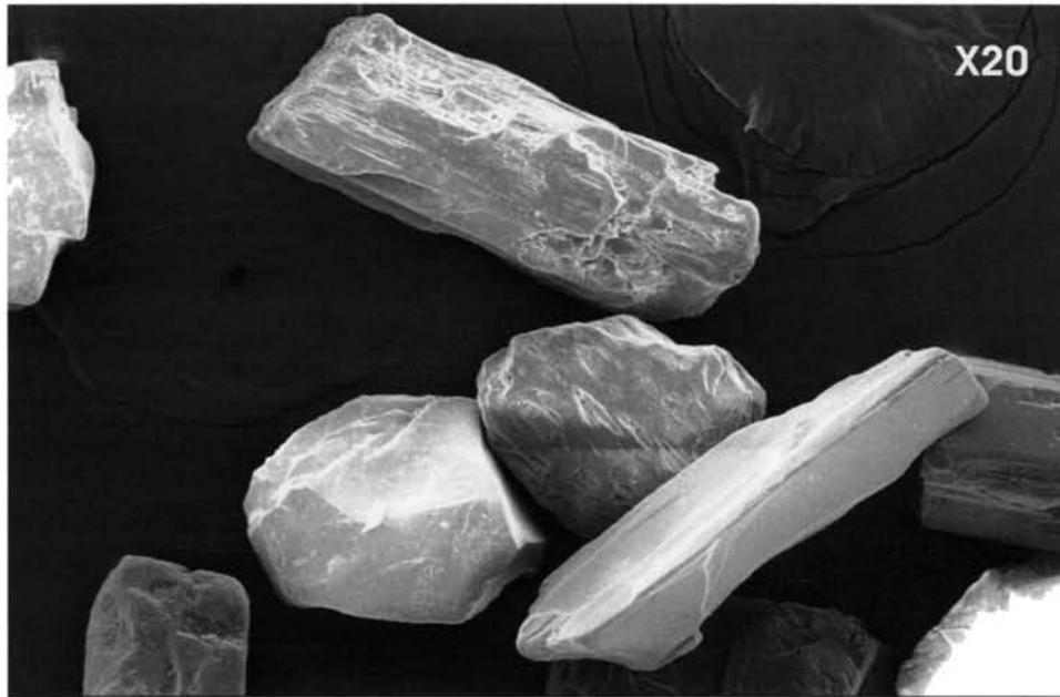
Plate 7k Scanning electron photomicrograph of hornblende in the fine sands collected at a depth of 0-50 cm in Pit 7 exhibiting elongated to subrounded step like grooves and chemical pits
