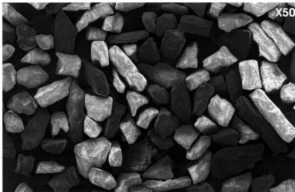
Plate 7d Scanning electron photomicrograph of some heavy minerals in the fine sands collected at a depth of 50-100 cm in Pit 18 showing angular to subhedral grains
