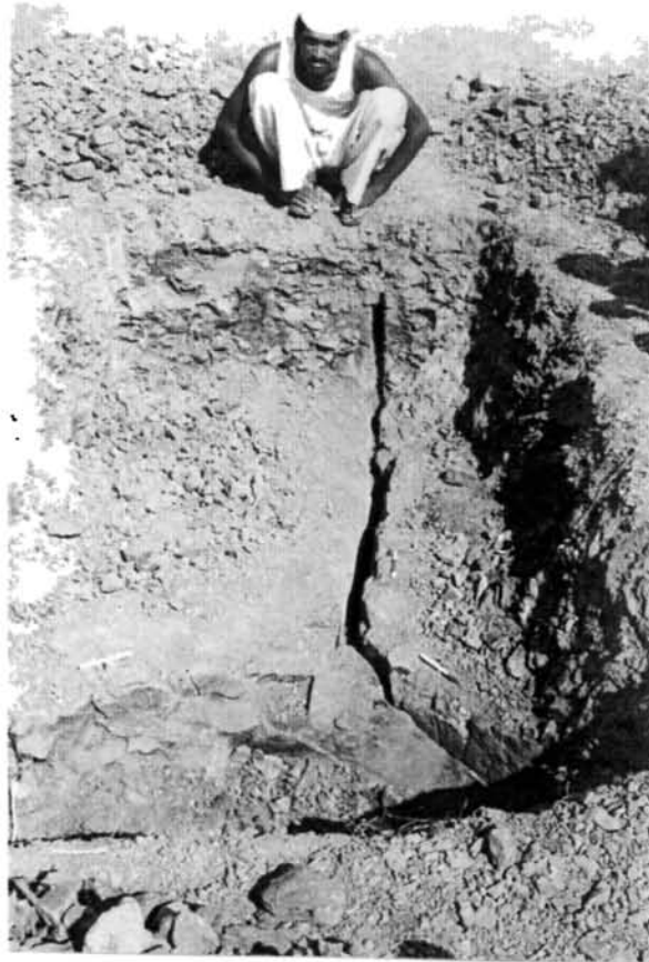
Fig. 4.7b. Photograph of the trench on the northern side of the surface rupture (courtesy: Pande, P). Note the compactness of the top layer of basalt compared to the rupture zone and its southern side.
