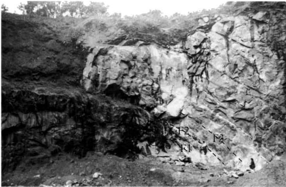
Fig. 6.2a. Photograph showing the quarry in which the fault is identified. The zone comprises a fault 'F2' and two sub parallel fractures 'F1 and F3', as represented in Fig. 6.3.
