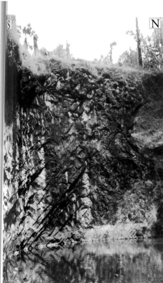
Fig. 5.7a. Photograph of a quarry section showing systematic joints developed in the hillock. These joints are parallel to the foliation direction.
