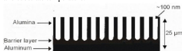
Fig. 1 Anodized aluminum sketch showing the barrier layer with the nano porous template.
