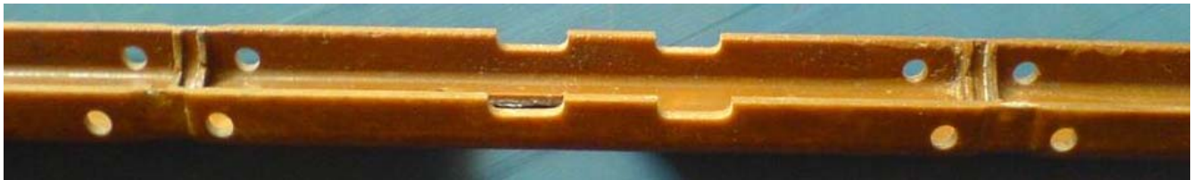
Figure 1: Section of the 'C' channel structure showing geometrical discontinuities
