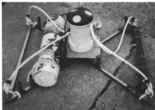
Fig. 2.6 Acoustic Doppler Current Profiler and battery pack fixed on a frame
