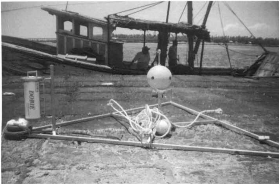
Fig. 2.4 S4 Current meter (spherical yellow colour) attached to stainless steel frame. The Dobie wave gauge is also seen attached to the same frame at one corner.
