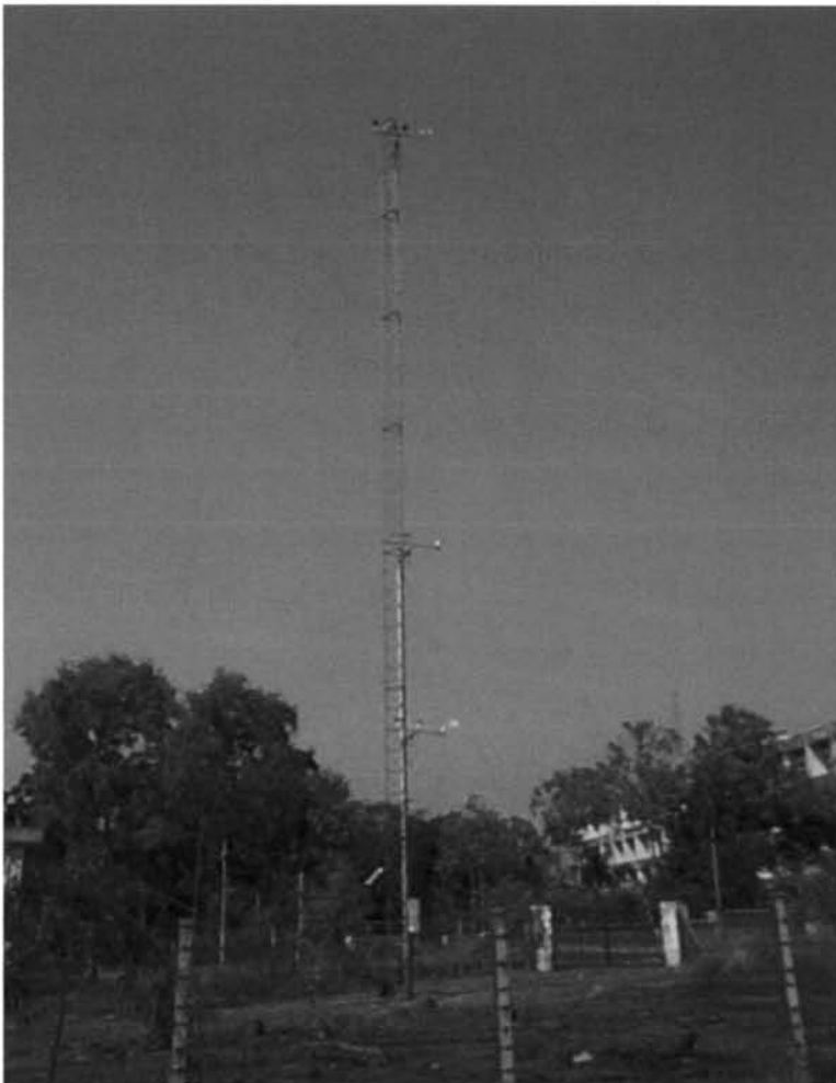
Fig.2.2 Micrometeorological Tower of 20 m height with three levels of sensors installed at Cochin University Campus for atmospheric boundary layer studies
