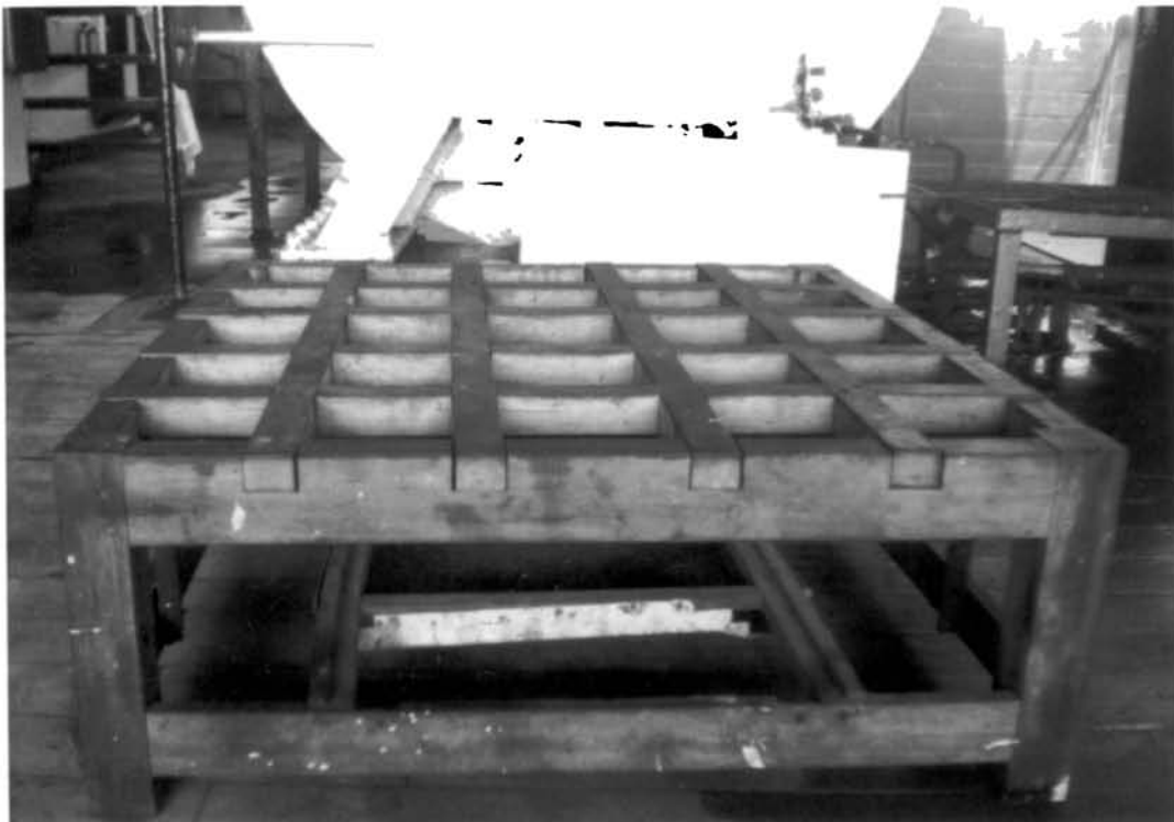
4B. Wooden platform for transferring & sieving sediment.
