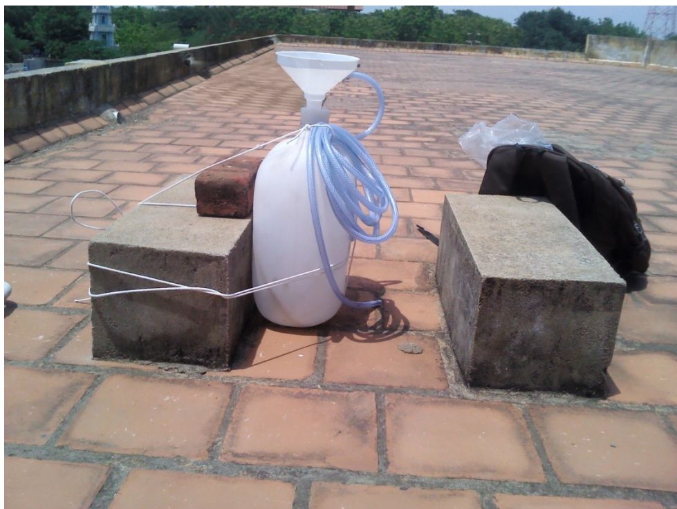
Plate 2.6: Rainwater collection unit for stable isotope investigation
