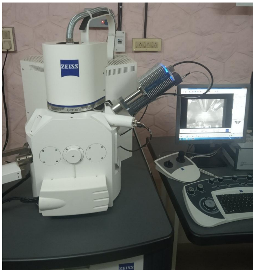
Fig. 3.7 FE SEM analysis set up
