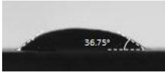
Figure 4.15 Contact angle measurement of SCN110.
