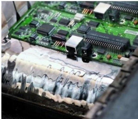
Fig. 1.5 Wave soldering process
