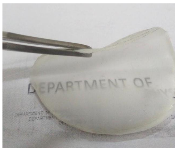
Figure 1: Transparent, flexible and freestanding SPE film
