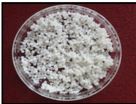
Plate 5.6: TiO 2 nanoparticles entrapped calcium alginate beads
