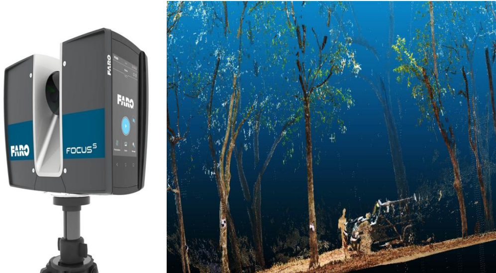
Figure 3.14: TLS Equipment and the Data Collected
