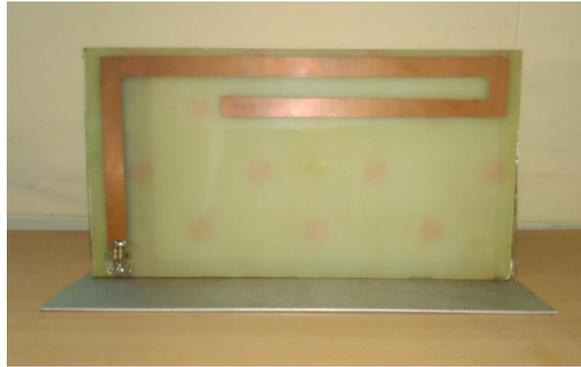
Fig 2.4. Photograph of a fabricated antenna.
