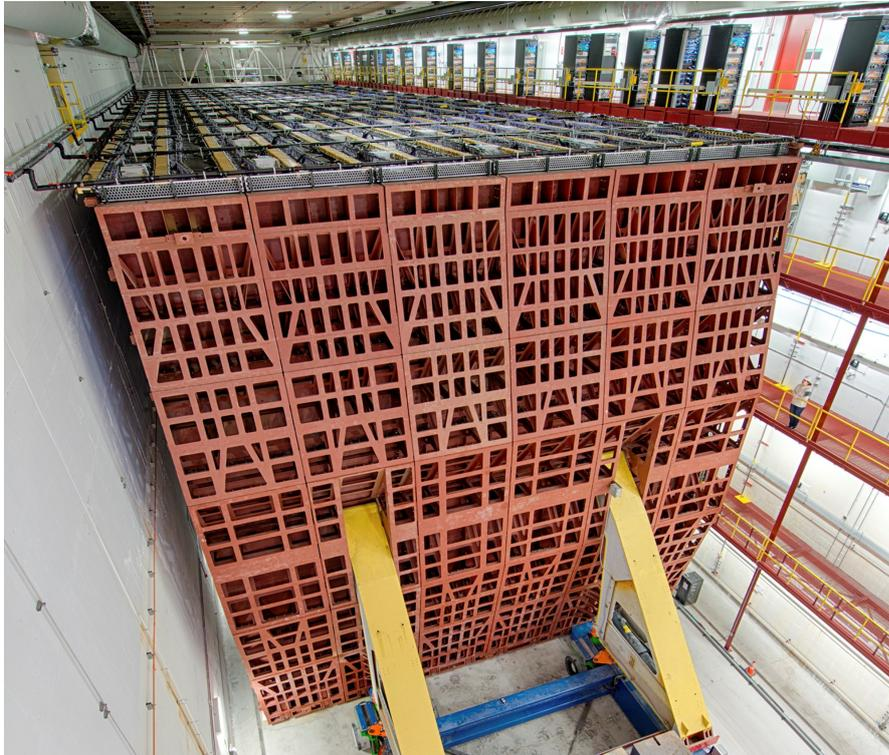
Figure 3.8: NOvA far detector. The beam comes from the back of the photograph and out of the page. The red and yellow structure is a pivoter used, not a part of the detector.
