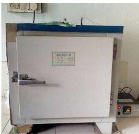
Figure 2.1. Oven used for the solvothermal synthesis of samples under study.
