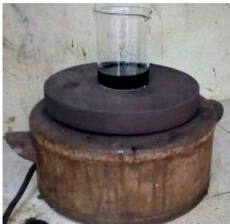
Figure 2.3. Heater used for the combustion synthesis of samples under study.
