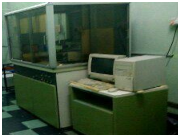
Figure 2.4. Rigaku Geigerflex D Max diffractometer with CuK \alpha radiation ( \lambda=1.5414 \text{ \AA} ) used for the analysis of some of the samples under study.
