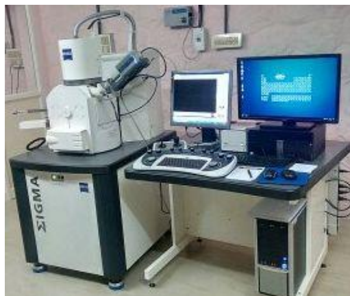
Figure 2.7. Carl Zeiss Sigma FE-SEM used to record SEM images of some of the sample under study.
