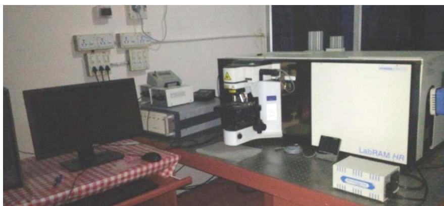
Figure 2.6. Horiba Jobin Yvon Lab RAM HR system used to record the Raman spectra of samples under study.
