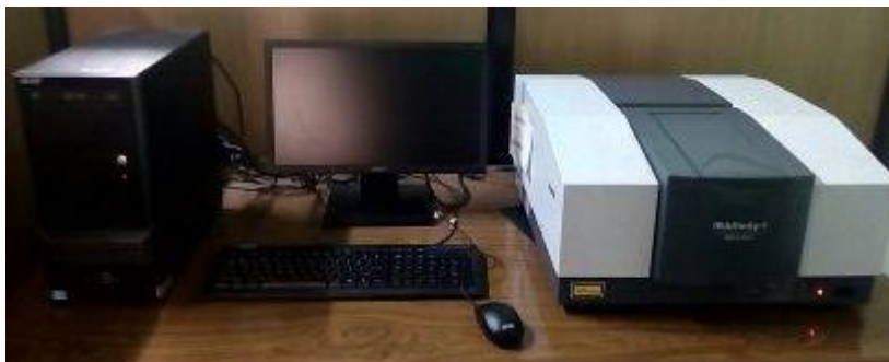
Figure 2.5. Shimadzu IR Affinity-1 FTIR spectrophotometer used to analyze the samples under study.
