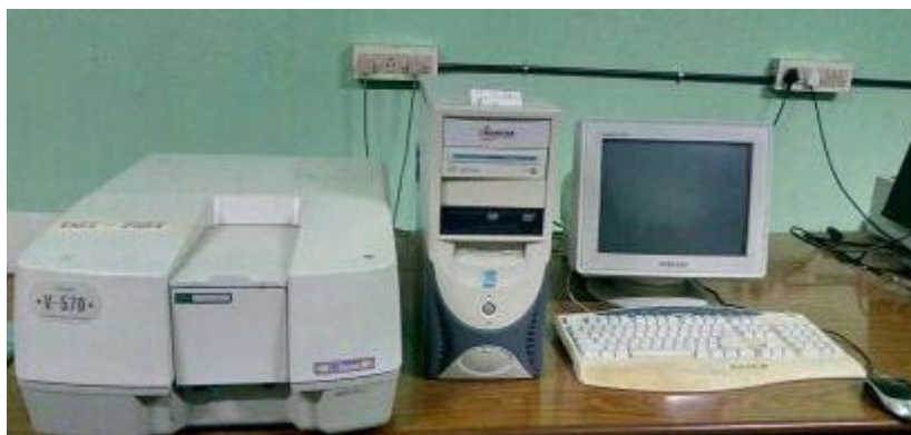
Figure 2.8. JASCO V 570 spectrophotometer used for the analysis of samples under study
