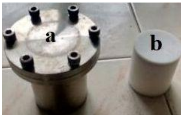
Figure 2.2. (a) Auto-clave (b) Teflon lined beaker used for the solvothermal synthesis of samples under study.
