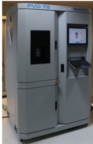
Fig. 2.13: Photograph of PVD-75 physical vapour deposition unit for the low temperature evaporation of pentacene.
