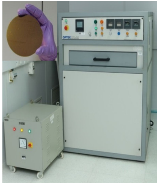
Fig. 2.7: Photograph of DPL-24 differential pressure laminator with the inset showing the polyimide film laminated silicon wafer.
