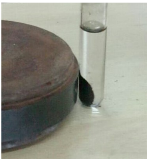
Figure: 2.18 Demonstration of magnetic separation of immobilized \alpha -amylase on CSM composite
