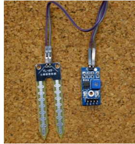
Figure A.2: Soil Moisture Sensing Unit with Electronic Board
