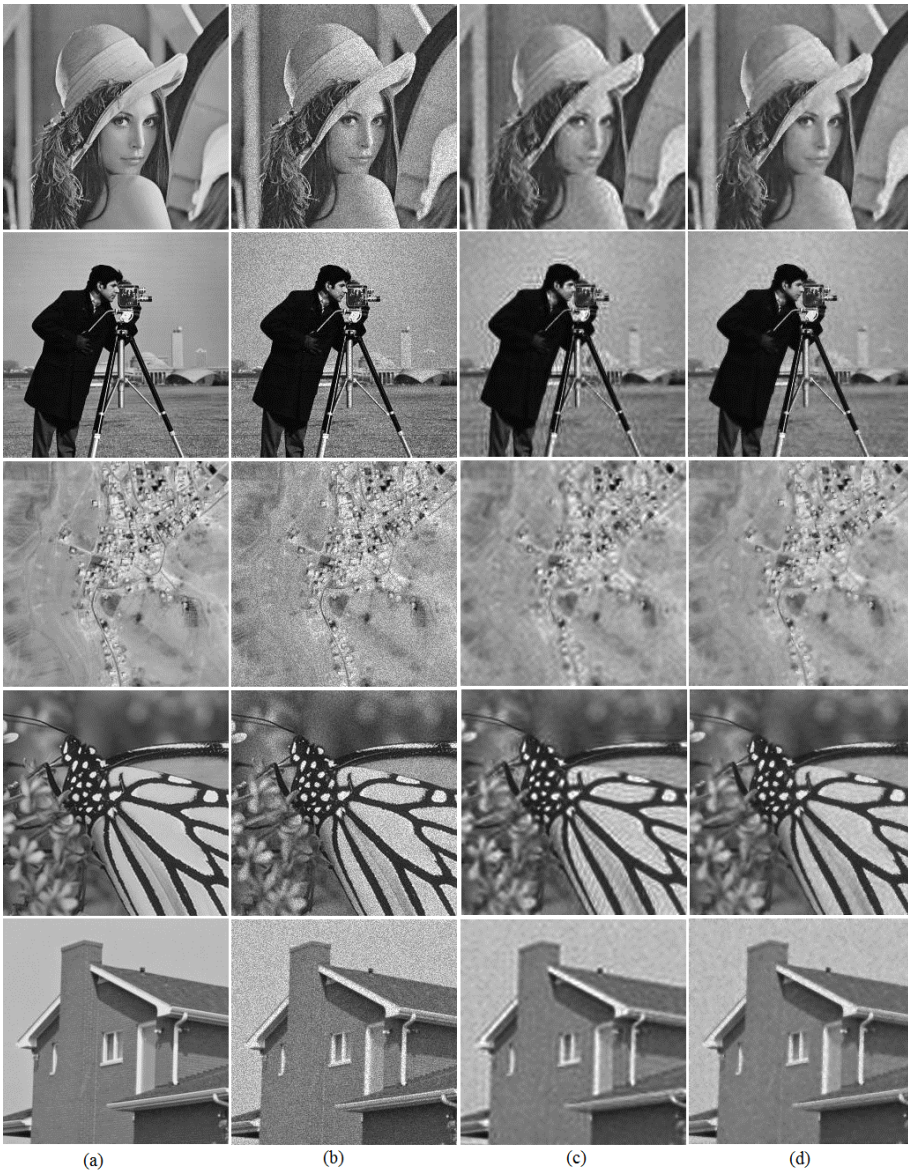
Figure B.2: (a) General images( lena , cameraman , egypt , monarch , house ) (b) images mixed with speckle noise variance of 0.01 (c) despeckled images by (Liu et al., 2014) (d) despeckled images using proposed algorithm
