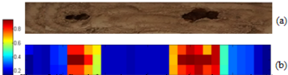
Figure 5.40: Result for moisture detection using colour-mapping (a) Camera shot (b) Colour-map; Sensor Antenna Method
