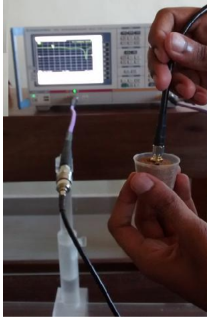
Figure 5.3: Experimental setup for measuring percentage shift in frequency for soil characterization; Sensor Antenna Method
