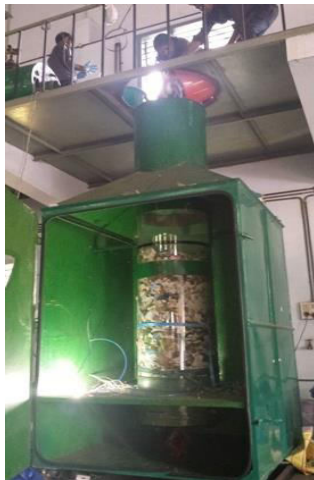
Filling the Biodrying Reactor
