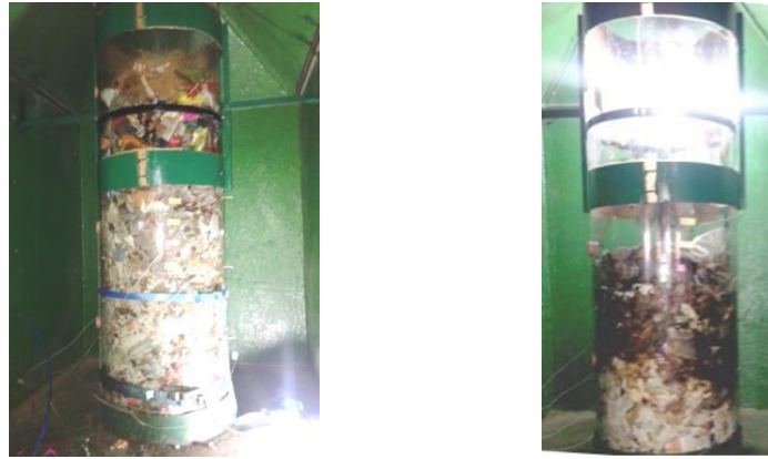
a) Filled Reactor Before Biodrying b) Biodrying Reactor After Process
