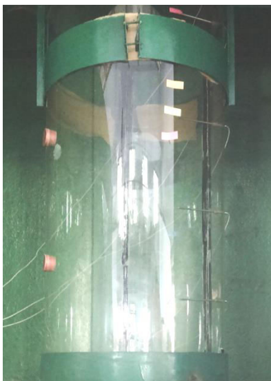
Fig. 5.2.2 Temperature Probes Inserted into the Biodrying Reactor.
