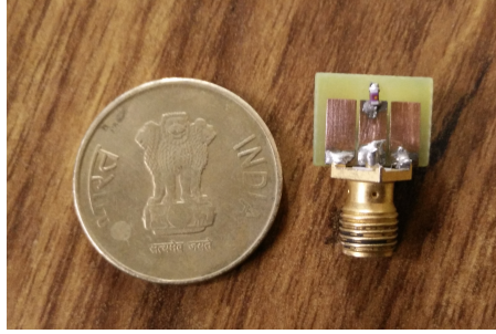
Figure 3.9: Prototype of the proposed antenna. [ \epsilon_r = 4.4 , P_h = 0.8 mm, P_w = 1 mm, G_w = 3 mm, Coilcraft 0603CS 23 nH Chip Inductor, S_h = 1.6 mm ]
