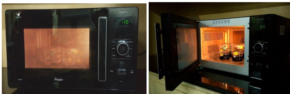
Fig. 3.2: Microwave reactor assembly: A) MW oven, B) Reaction samples inside the oven
