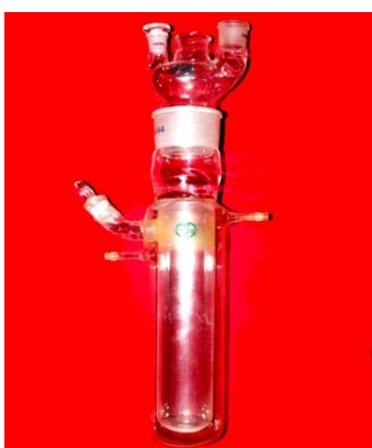
Fig. 3.3: Inhouse designed MW/photocatalytic reactor
