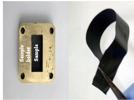
Fig. (8b) Schematic diagram of the Fig. (8c) Sample holder and sample set-up
