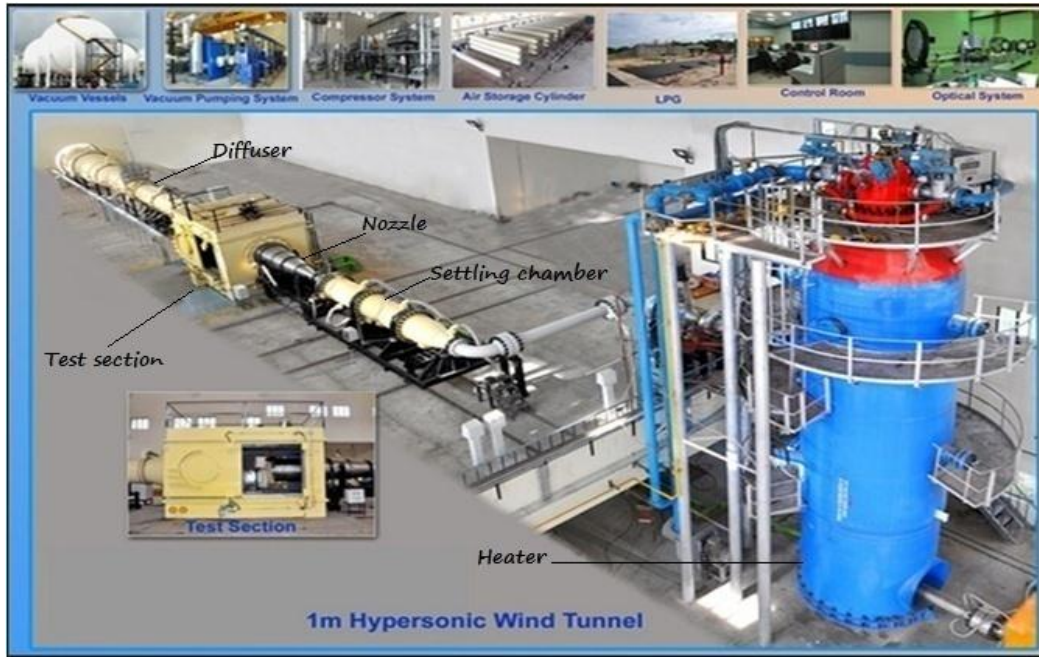
Fig.1.5 1 m Hypersonic Wind Tunnel in VSSC, Trivandrum – Mach number 6 (Vikram Sarabhai Space Centre, VSSC)
