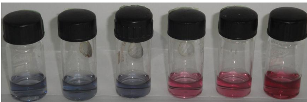
Figure 7.11: Photographs of a solution of (1) AuNPs + 1 \times 10^{-4} M TET, (2) AuNPs + 5 \times 10^{-5} M TET, (3) AuNPs + 1 \times 10^{-5} M TET, (4) AuNPs + 5 \times 10^{-6} M TET, (5) AuNPs + 1 \times 10^{-6} M TET and (6) AuNPs in the presence of 2.5 \times 10^{-5} M \text{Cu}^{2+} (from left to right)
