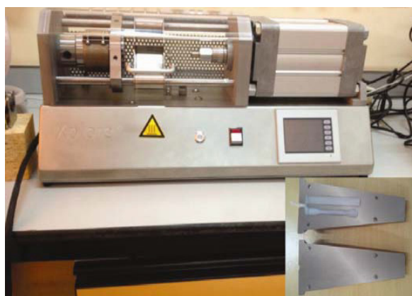
Figure 2.6. Semi micro injection molding machine
