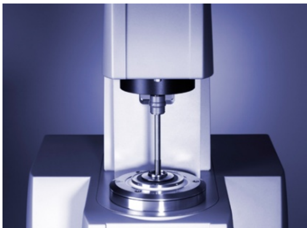
Figure 2.11. Parallel plate rheometer (MCR 102)
