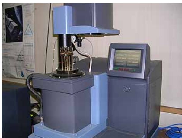
Figure 2.12. Dynamic mechanical analyser
