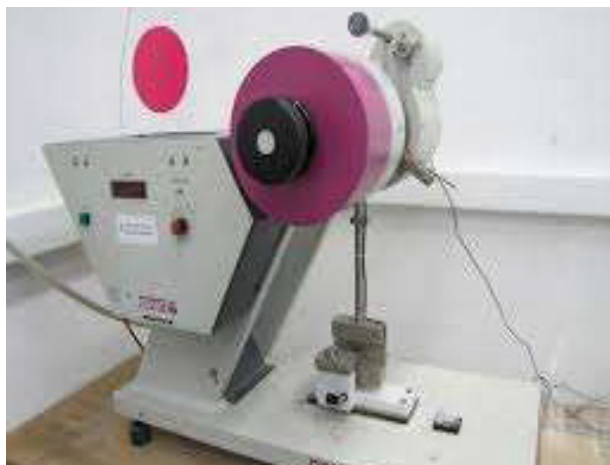
Figure 2.10. Impact tester (RESIL)
