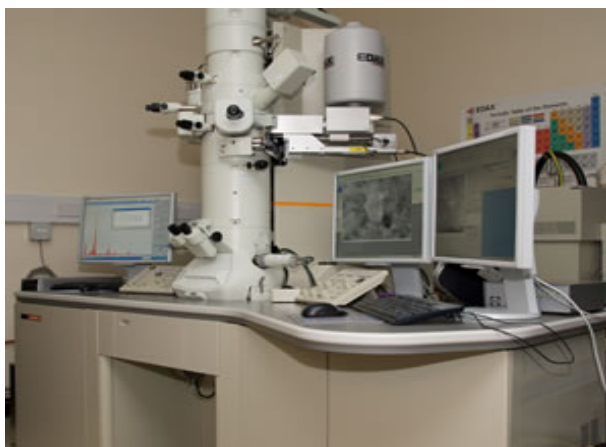
Figure 2.8. Transmission electron microscope
