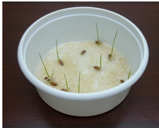
Figure D4. 4: O. sativa grown in grown in 20% zeolite in OECD sediment.
