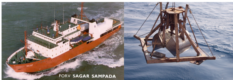
Fig. 2.4. Sampling platform FORV Sagar Sampada and sampling gear Smith McIntyre grab
