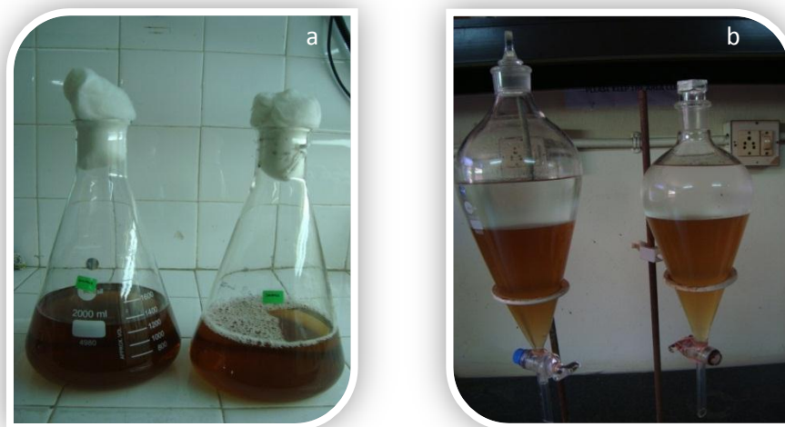
Fig. 7.2: a) Mass production and b) Ethyl acetate extraction of Pseudonocardia sp. MCCB 268
